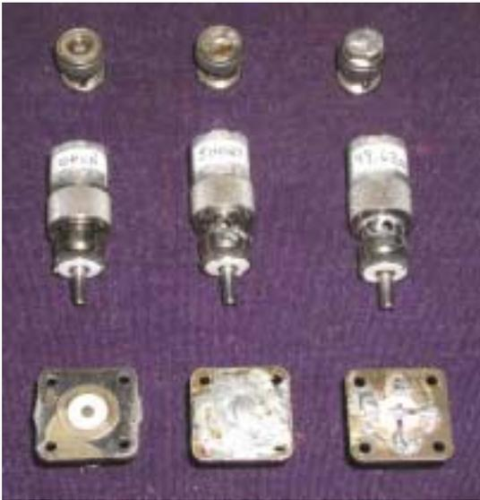
The Load standard is typically a nominal 50-ohms, but can be 25 to 100 ohms with little loss in accuracy as long as the “Rstd” parameter in the “Rocky.ini” file is assigned the actual resistance value. See the next section for more about Rstd.
